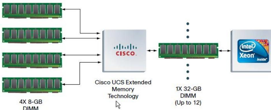
**CISCO EXTENDED MEMORY TECHNOLOGY MAKES FOUR PHYSICAL DIMMS APPEAR TO THE CPU AS A SINGLE, LARGE, LOGICAL DIMM**
