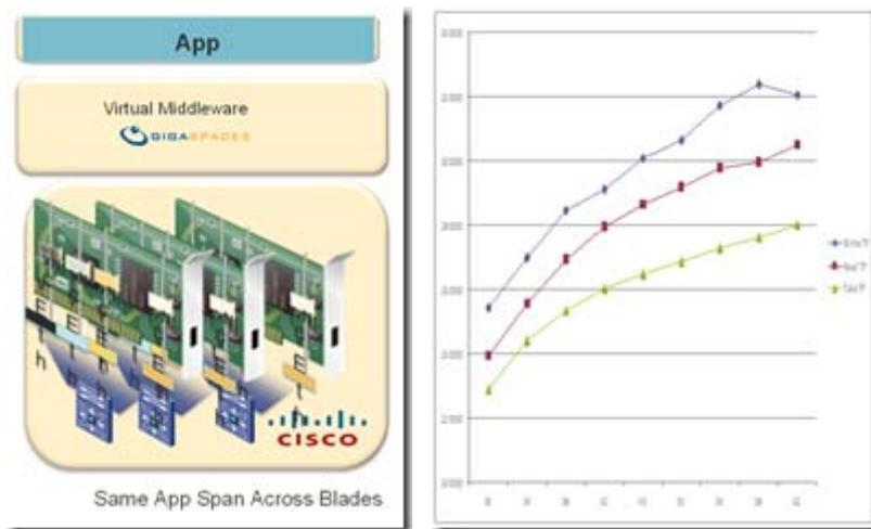
The diagram above illustrates the linear system scaling that occurred as the number of concurrent clients grew. The system reached approximately 320,000 operations/sec. A detailed analysis is provided below.
